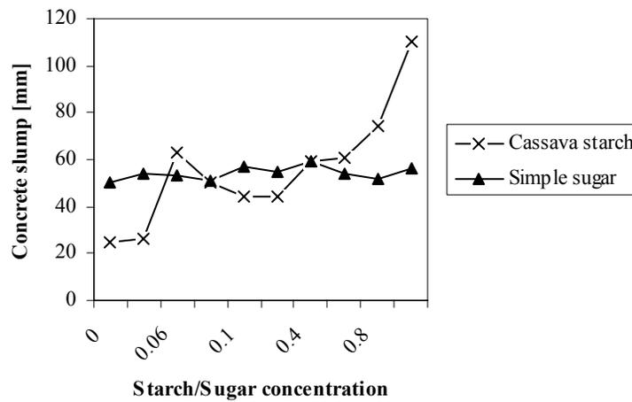
Figure 6. Effect of cassava starch and sugar on slump of fresh concrete.
