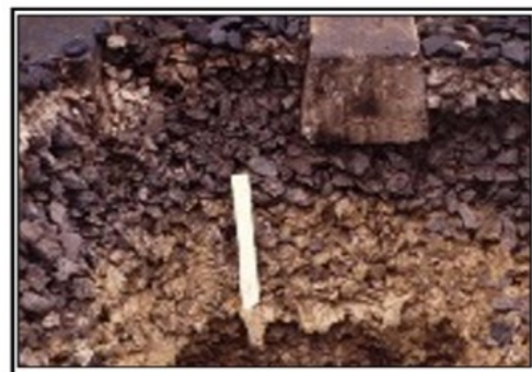
Figure 10: Fine materials migrating upwards
