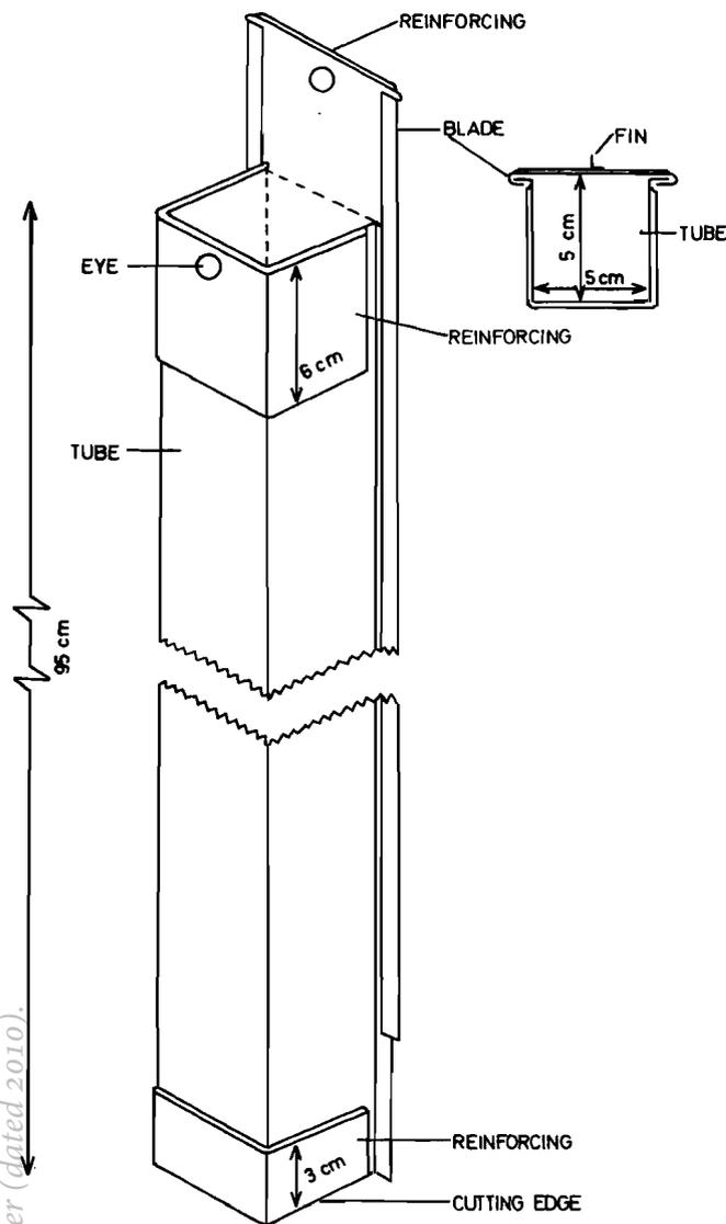
Fig. 1 Diagram of the corer showing the interlocking blade.
