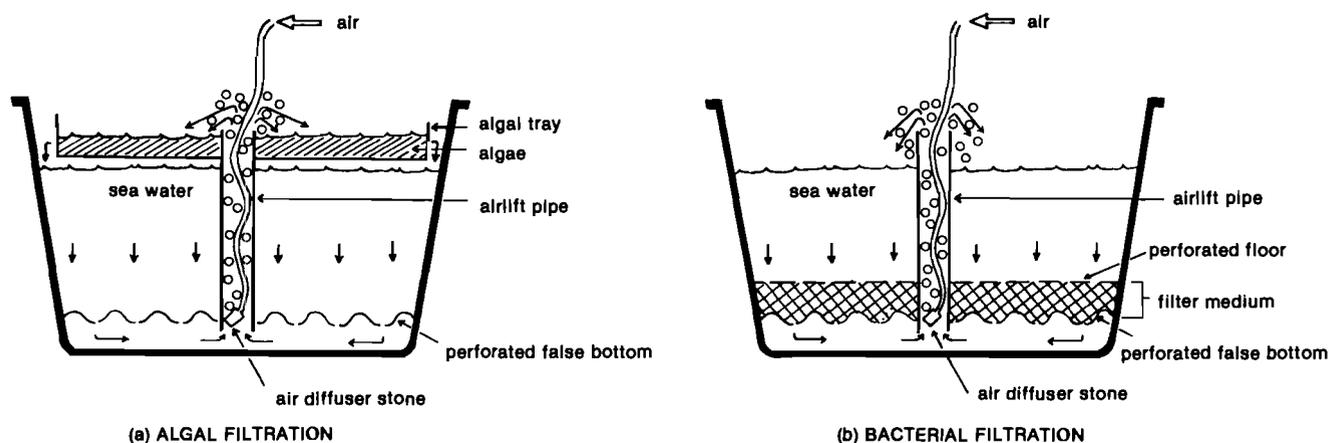
Figure 1 Diagram of (a) an algal filtration system and (b) a bacterial filtration system used in the experimental trials. Arrows indicate the direction of water flow.
