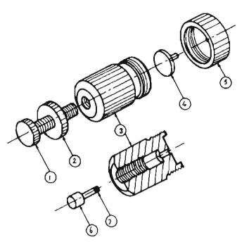
Figure 1 An isometric and exploded view of the mould with plunger (6,7), screw and locknut (1,2), body (3), stub (4) and stub retainer (5). Diameter of body 20 mm, length of body 27 mm.
