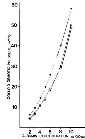
Figure 2 C.O.P. of albumin solutions obtained with the concentrator  $(\Delta - \Delta)$ , Prather *et al.* osmometer  $(\Delta - \Delta)$  and by calculation  $(\bullet - \bullet)$ . For clarity S.D. is not shown (n = 6 for each set of measurements).
