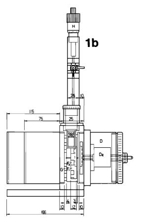
**Figure 1b** Side view of respirometer to show the position of the electric motor (D), impeller (F) and KOH absorption vial (M).
