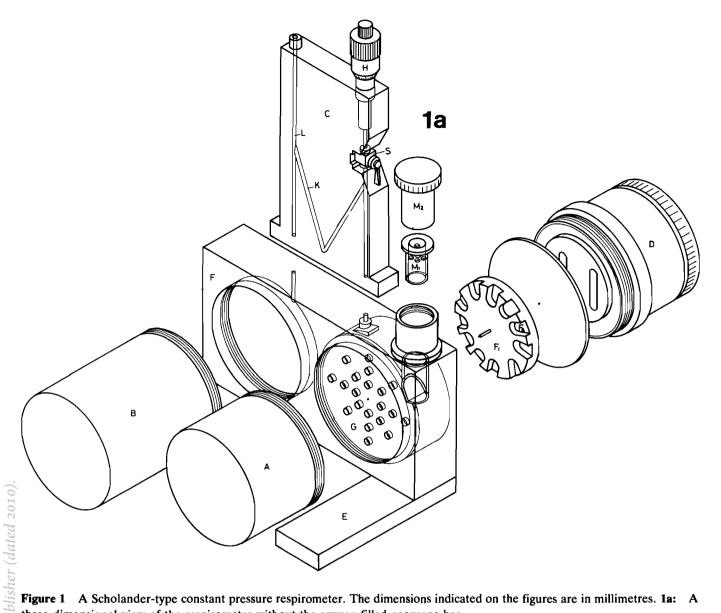
Figure 1 A Scholander-type constant pressure respirometer. The dimensions indicated on the figures are in millimetres. 1a: A three-dimensional view of the respirometer without the oxygen-filled neoprene bag.
