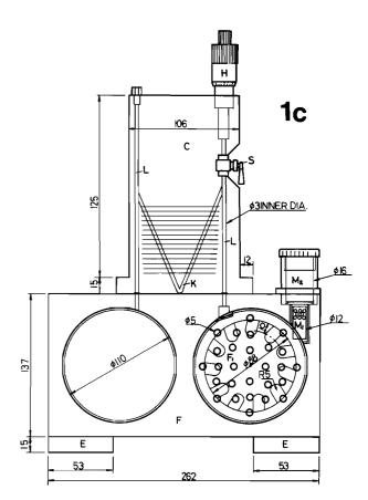
Figure 1c Front view of respirometer without respiration chamber (A) and compensation chamber (B) to show the pattern of the notched holes (F) on the impeller.
