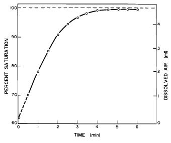
**Figure 2** A graphical representation of the rate of gas absorption into 62% saturated water at 25°C. The impeller wheel was rotated at a speed of 200 rpm to mix the degassed water (341 ml) with the gassed water (559 ml).
