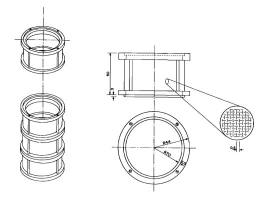
Figure 1 Three dimensional and technical drawings of the segments of the moisture towers constructed for the preference studies.
