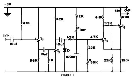
The circuit for the "radiation alarm". Modified from Inglis et al. 1968 ( $T_1$ ,  $T_2$ ,  $T_3$  and  $T_4 = OC 71$ ; D=OA 85).
