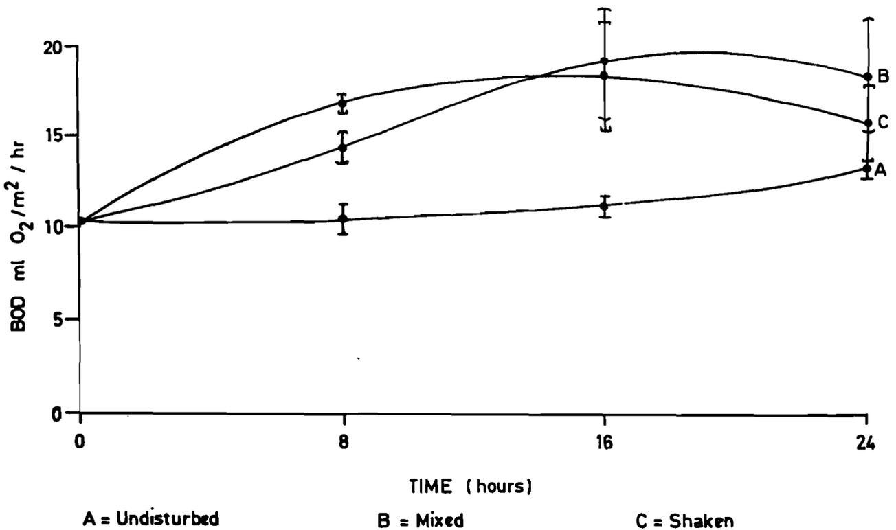
Fig. 2 The effect of disturbance on BOD as measured in incubated cores.
