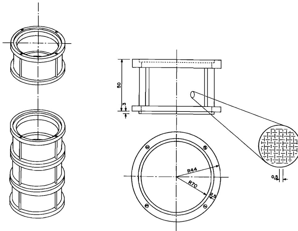
**Figure 1** Three dimensional and technical drawings of the segments of the moisture towers constructed for the preference studies.
