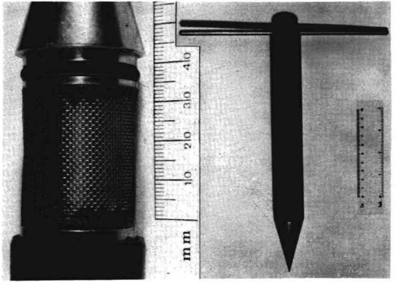
FIGURE 2 Coring device for obtaining interstitial water in fine substrates.
