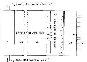
Fig. 1 Top view of gradient apparatus. D{ Distributor, showing arrangement of the two supply tubes. GC: Gradient chamber. MR: Mixing region filled with glass balls. OB: Outflow baffle, showing arrangement of outflow tubes, OT. Snails were placed between zones IV and V before securing the water-tight lid.
