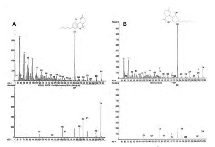
**Figure 2** GC/MS chromatograms showing that the cannabis vapor extract contains (A)  $\Delta^9$ THC and (B) cannabidiol.
