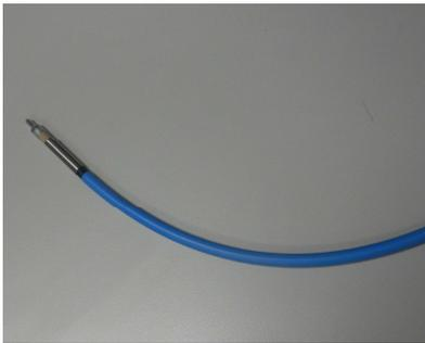
**Fig 1:** PTW-Waterproof PinPoint chamber used for depth dose and absolute dose measurements.
