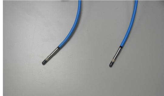
**Fig 2:** PTW-Waterproof Semiflex chamber used mainly for dose distribution measurements in motorized water phantoms.
