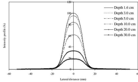
**Fig 7:** The beam profiles measured using semiflex chamber for smallest field size 2x2 cm at different depths; 1.6, 3, 5, 10, 20, and 30-cm.
