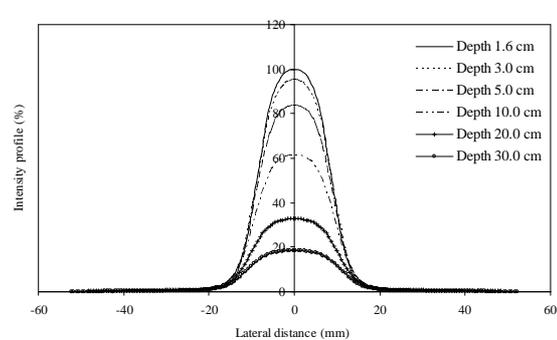
**Fig 6:** The beam profiles measured using PinPoint chamber for smallest field size 2x2 cm at different depths; 1.6, 3, 5, 10, 20, and 30-cm.
