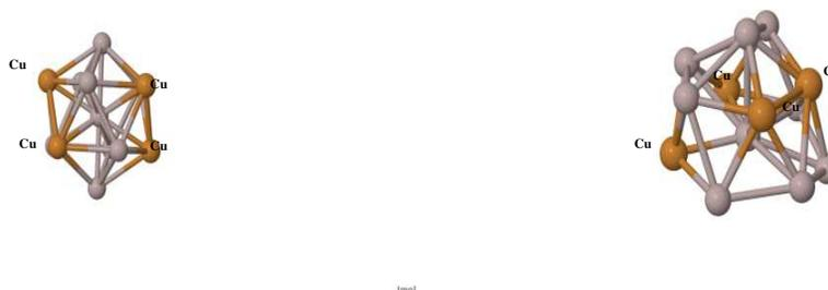
**Figure 11: Geometry of  $Al_9Cu_4$  (a) Before relaxation and (b) After relaxation (produce by Jmol molecular viewer)**
