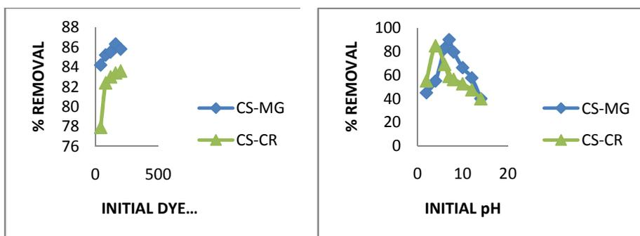
Figure 2. Effect of (a) initial dye concentration and (b) pH against % removal of MG and CR dyes.
