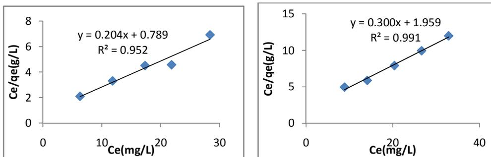
Figure 5: Langmuir isotherm (a) CS-CR and (b) CS-MG
