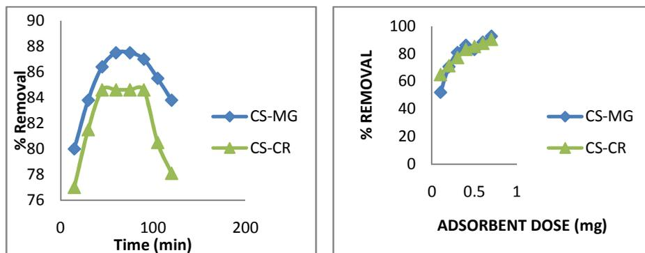
Figure 1. Effect of (a) time and (b) adsorbent dose on the percentage removal of MG and CR dyes
