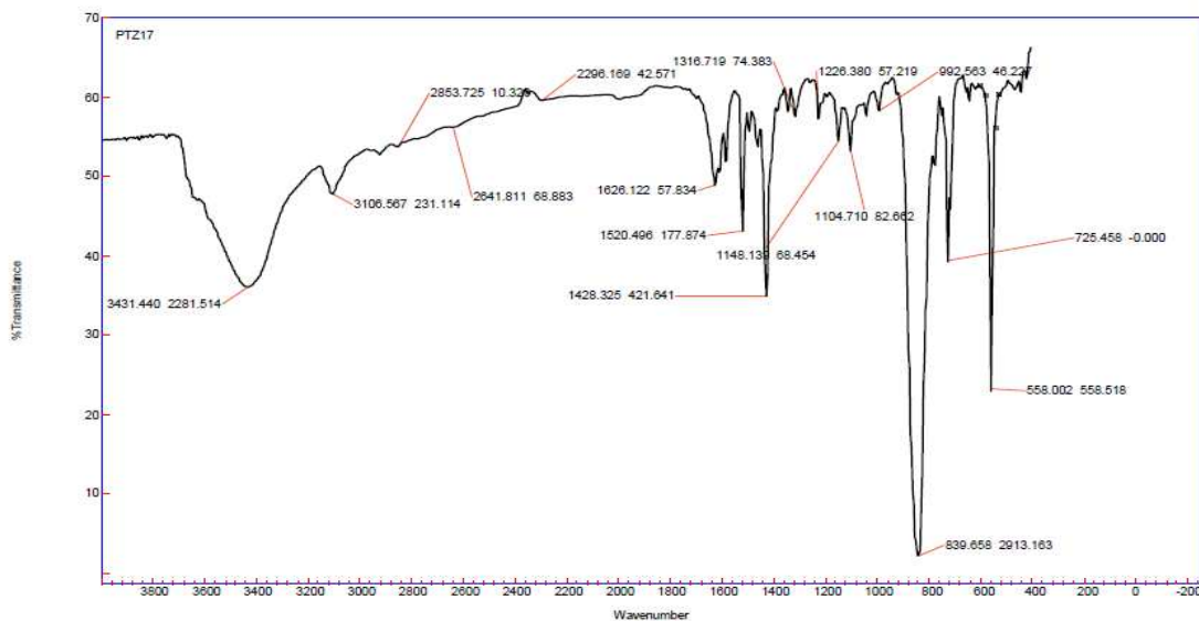
Fig.3: IR Spectrum of [Ru(bpy)_2PDB](PF_6)_2
