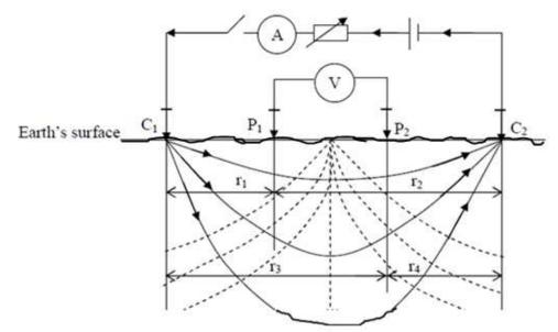
Figure 4: Current and Potential Distributions within Homogeneous Isotropic ground.
