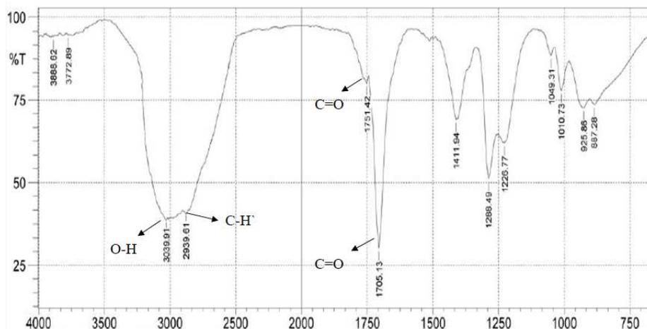
Figure 3: FT-IR Spectrum of LA produced from Groundnut shell
