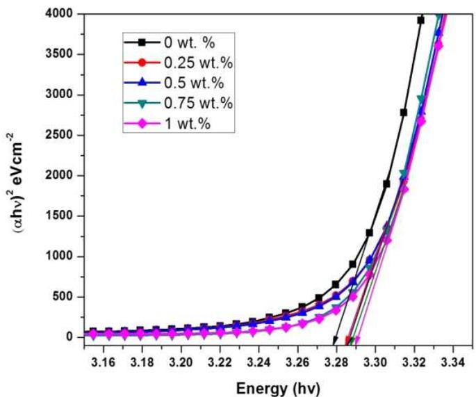
**Figure 3: Optical bandgap values for ZnO and Mo:ZnO thin films**
