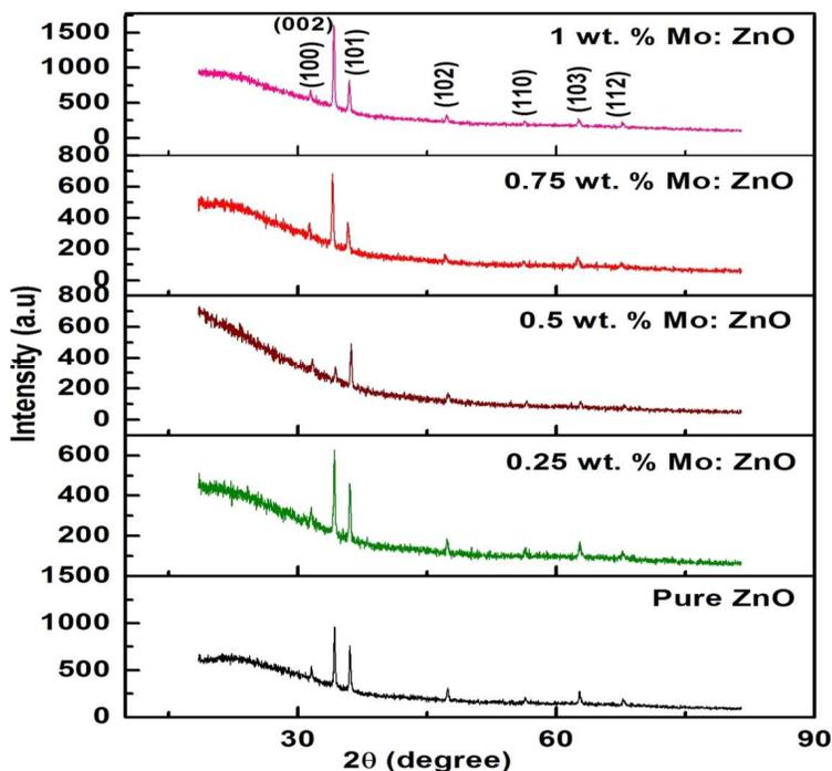
Fig.1. XRD patterns of undoped and Mo doped ZnO thin films.
