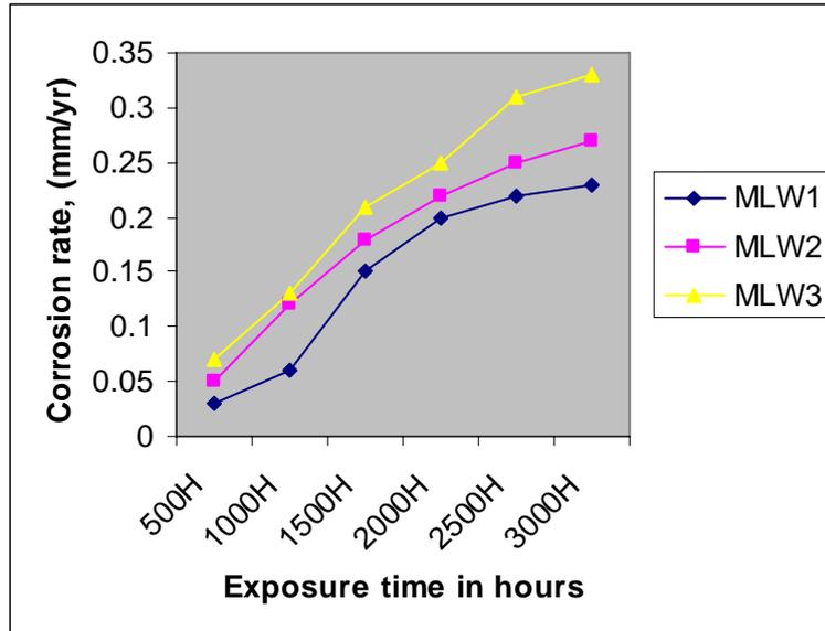
Figure 3: Corrosion rate of galvanized steel against exposure time in moving liquid waste samples collected within the core city.
