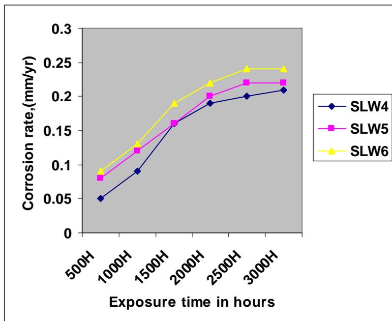
Figure 2: Corrosion rate of galvanized steel against exposure time in stagnant liquid waste samples collected outside the core city.
