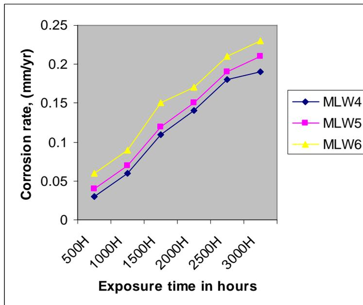
Figure 4: Corrosion rate of galvanized steel against exposure time in moving liquid waste samples collected outside the core city.
