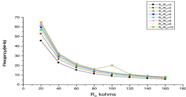
Figure 8.0 Graph of nominal Converter frequency for  $C_T = 1nF$
