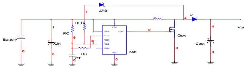
Figure 2.0 DC-DC Boost converter
