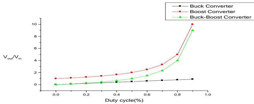
Figure 5.0 Graph of commonly converters compared analytically with equation 2.0 which shows the boost converter has high gain.
