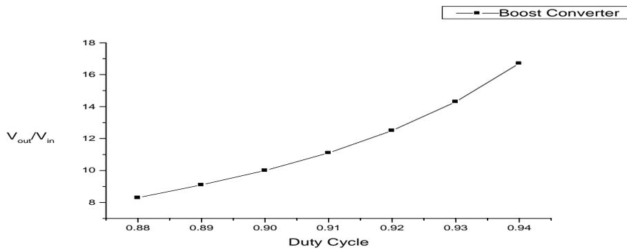
Figure 6.0 Graph of the gain to the duty cycle from the simulation result
