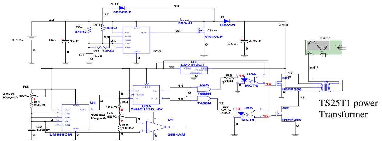
Figure 14. DC-DC/DC-AC power Inverter stage
