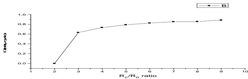
Figure 7.0 Graph of maximum duty cycle with ratio of timing resistors  $R_C/R_D$
