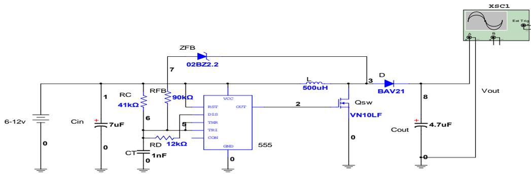
Figure. 13 DC-DC converter stages with the nominal calculated values
