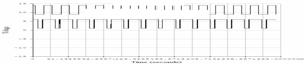
Figure 11.0 Output wave form for the two AND-gate
