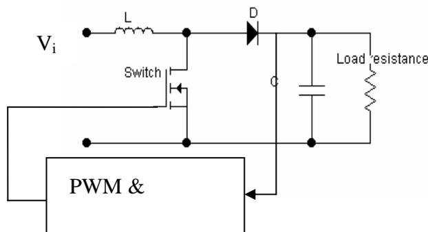
Figure 1.0: Boost converter schematic diagram
