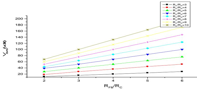
Figure 9.0 Graph of Bias voltages plot from equation (3.7)
