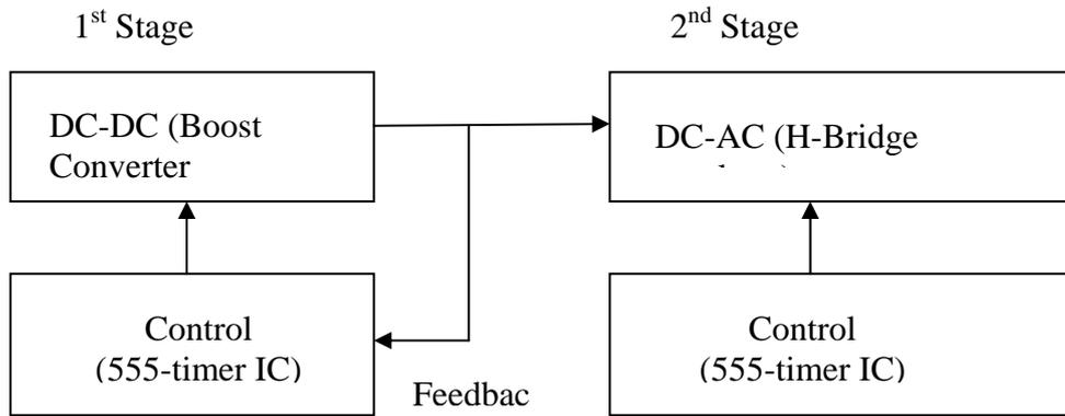
Figure 4.0 DC-AC Inverter circuit design
