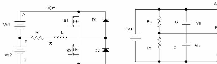
Figure 3.0 (i) Half-bridge inverter with dual supply, and (ii) single supply
