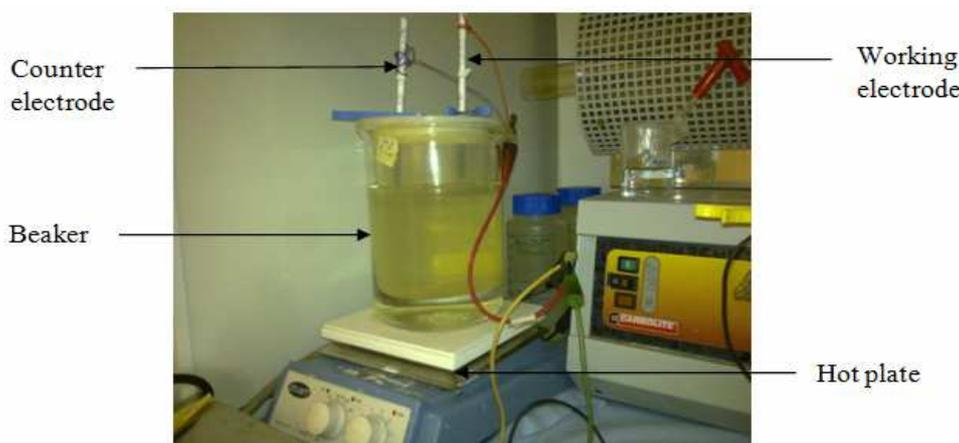
**Figure 10 (b):** A photograph of a typical two electrode set-up.
