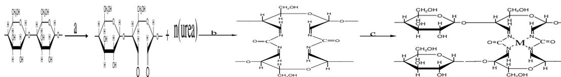
Scheme 1: Synthesis of dialdehyde starch urea complex from starch; (a) NaIO<sub>4</sub>; (b) ethanol; (c) Co(II), Pb(II) or Zn(II) salts
