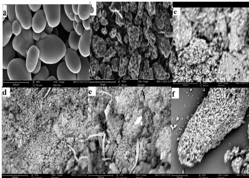
Fig. 7: Photomicrograph of (a) Starch granules X 380 (b) DAS X 1000 (c) DASU X 1000 (d) DASU-Co X 255 (e) DASU-Pb X 255 (f) DASU-Zn X 500.
