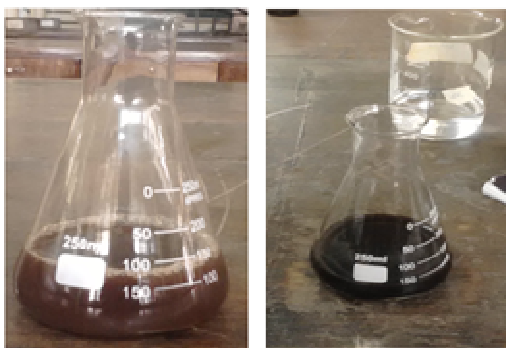
(a) (b) Fig. 1: Formation of AgNPs detected by the colour change. (a) Plant sample extract without \text{AgNO}_3 Solution and (b) Plant Sample extract with \text{AgNO}_3 Solution.
