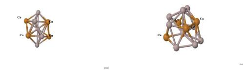
Figure 11: Geometry of  $Al_9Cu_4$  (a) Before relaxation and (b) After relaxation (produce by Jmol molecular viewer)
