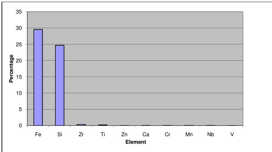
Fig. 2: Elemental Composition of Itakpe Iron Ore
