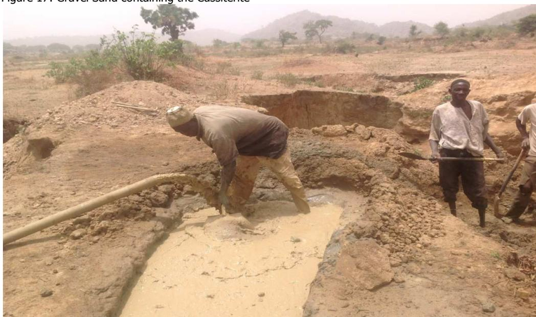
Figure 18: Local Separation of the Cassiterite from the gravel sand
