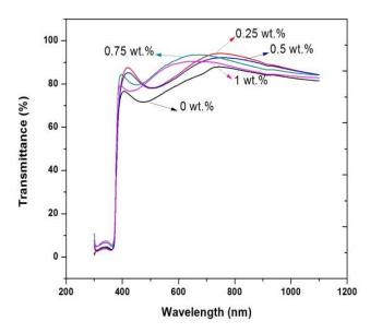
Figure 2: Optical transmittance of ZnO and Mo:ZnO thin films
