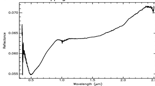
Figure 2. Laboratory spectrum of perovskite- bearing ilmenite (Kokaly *et al.*, 2017). Reflection peak and trough are identifiable at 2.4  $\mu\text{m}$  and 0.5  $\mu\text{m}$  respectively.
