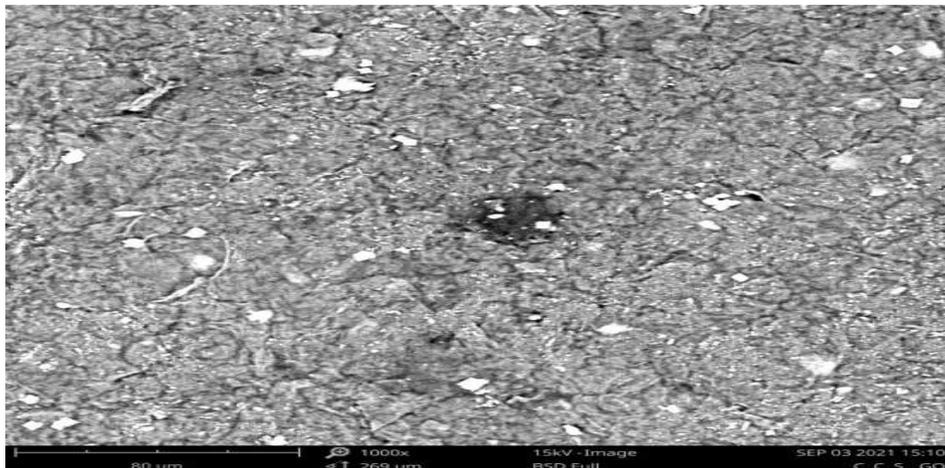
Figure 5: SEM image of composite adsorbent
