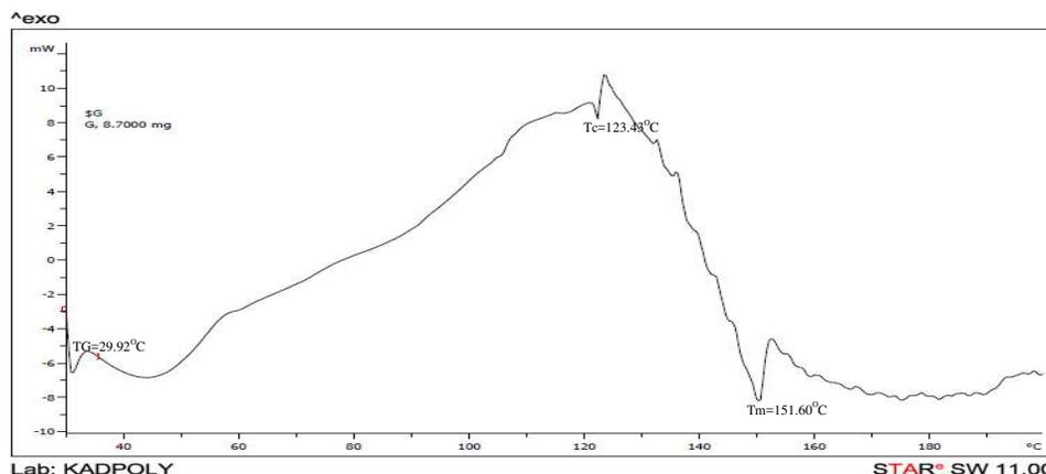
Figure 4: Differential Scanning Calorimetry Curve of CLS-GO
