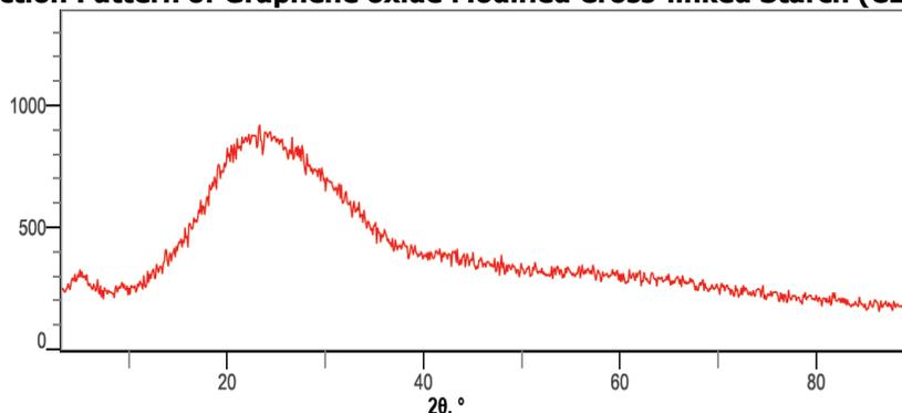
Figure 3: The XRD pattern of CLS-GO Composite adsorbent
