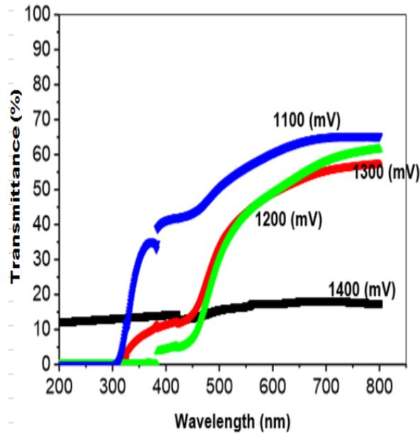
**Figure 2:** Graph of the transmittance versus wavelength at different growth voltages
