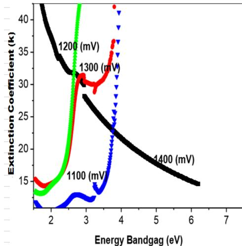
**Figure 5:** Graph of the extinction coefficient versus energy bandgap at different growth voltages.
