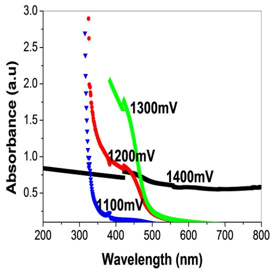
**Figure 4:** Optical absorbance curves for CdS deposited at different growth voltages.
