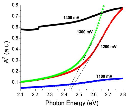
**Figure 1:** Optical absorption curves for CdS deposited at different growth voltages.
