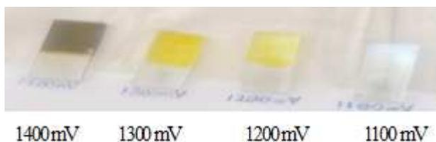
**Plate 1:** As deposited ED-CdS thin films on glass/FTO substrates of different growth voltage
