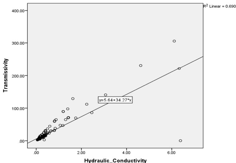
Fig. 4: Regression plot of Transmissivity against Hydraulic Conductivity
