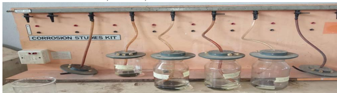
Fig. 1. Corrosion studies kit showing the metal samples in 3.5 % NaCl
