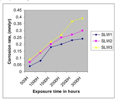
Figure 1: Corrosion rate of galvanized steel against exposure time in stagnant liquid waste samples collected within the core city.
