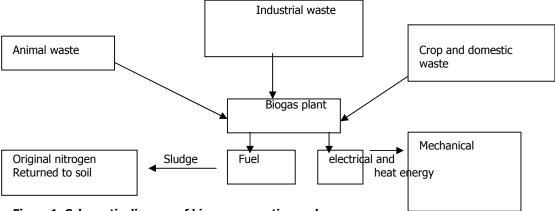
Figure 1: Schematic diagram of biogas generation and uses
