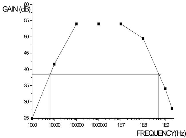
Fig 7.0.A graph of Gain (dB) Versus Frequency (Hz) For Distributed Amplifier
