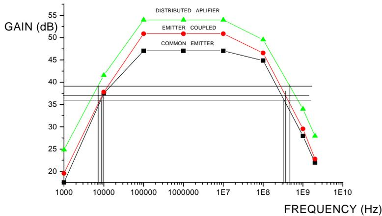
Figure 8.0. Comparison Graphs of Gain (dB) versus Frequency (Hz) for Common Emitter Amplifier, Emitter-coupled Amplifier and Distributed Amplifier.
