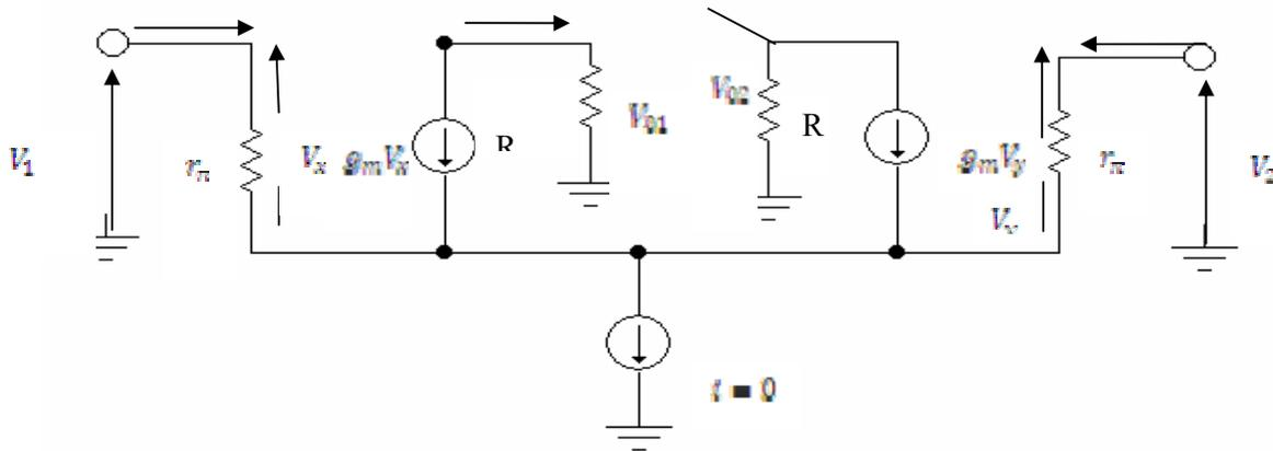
**Figure 3.0: Hybrid pi- model for Emitter- Coupled Amplifier**
