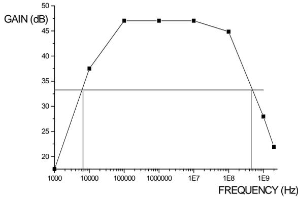
**Figure 5.0: A Graph of Gain (dB) versus Frequency (Hz) for Single Stage Common Emitter Amplifier**
