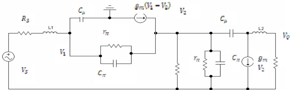
Figure 4.0: Hybrid pi- model of one of the amplifier element of the Distributed Amplifier
