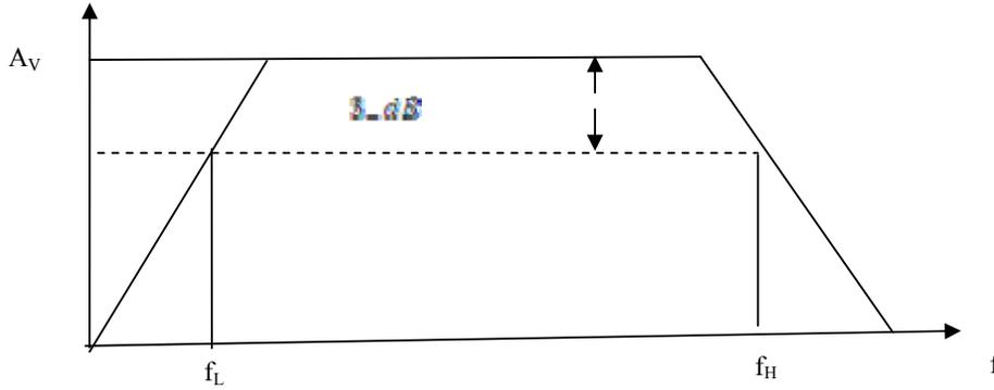
**Figure 2.0 A graph of Gain(dB) versus frequency(Hz)**
