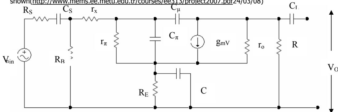
Fig 1.0 Common Emitter Amplifier Hybrid pi -model for low and high
