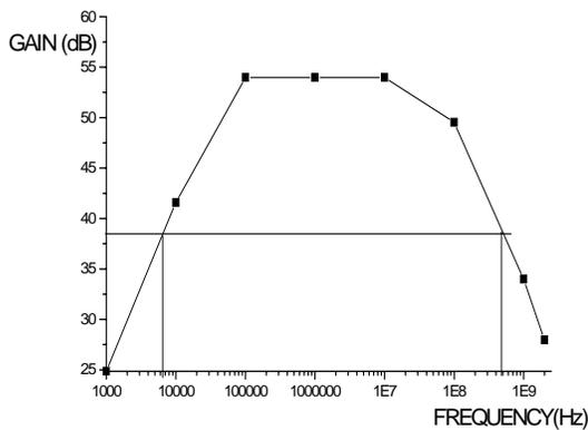
**Fig 6.0 A Graph of Gain (dB) versus Frequency (Hz) for Emitter- Coupled Amplifier**
