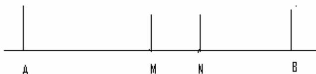
**Figure 1: Schlumberger Electrode array**
