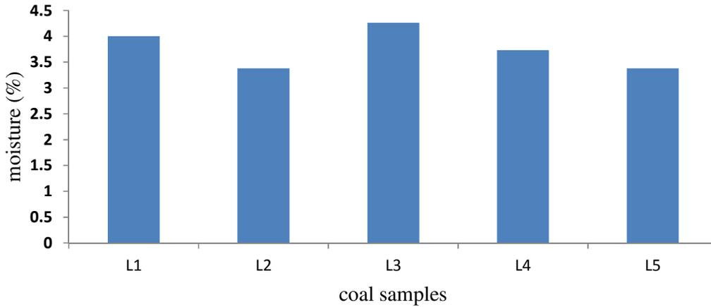
**Figure 1:** moisture content of Guyuk (Lamza) coal at different locations
