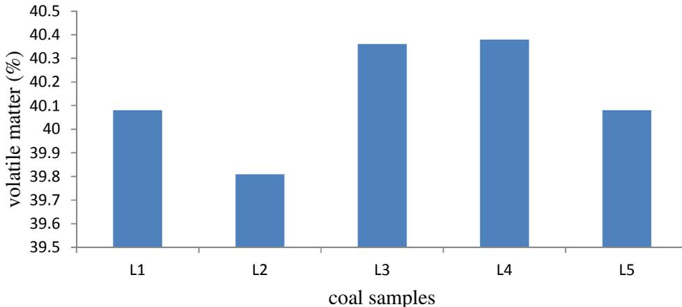
**Figure 3:** volatile matter of Guyuk (Lamza) coal at different locations
