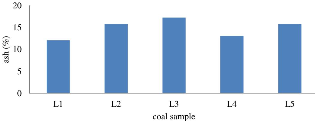
**Figure 2:** ash content Guyuk (Lamza) coal at different locations
