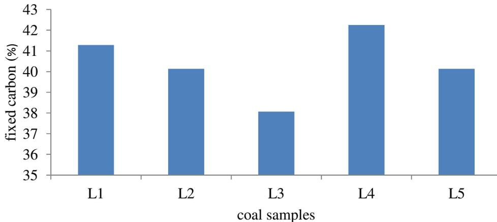
**Figure 5:** fixed carbon values of Guyuk (Lamza) coal at different locations
