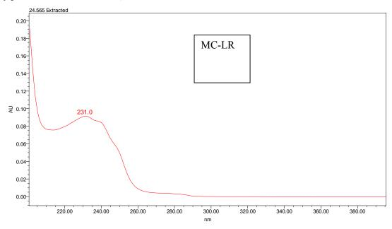
Figure 2: Absorption Spectra and retention time of Microcystin - LR as determined by HPLC-PDA
