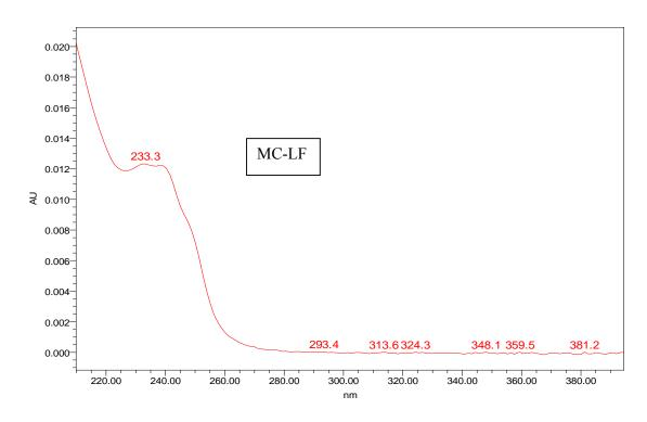
Figure 5: Absorption Spectra and retention time of *Microcystin* - LF variant as determined by HPLC-PDA
