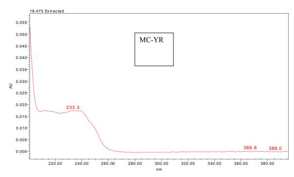
Figure 3: Absorption Spectra and retention time of *Microcystin* - YR variant as determined by HPLC-PDA
