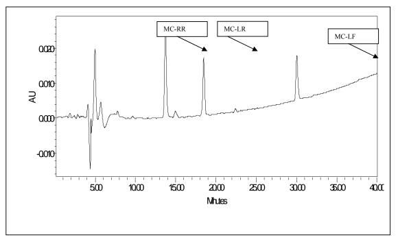
Figure 7: HPLC chromatograms of the toxin variants (MC, RR, LR and LF) detected and identified in *M. aeruginosa* isolates from six burrow pits in Kano metropolis
