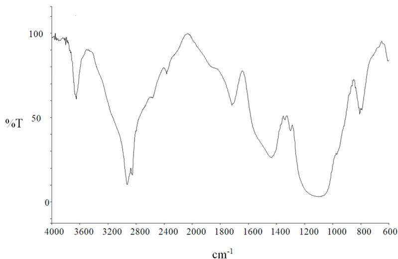
Figure 3. IR spectrum of a typical thiol-silica composite material.
