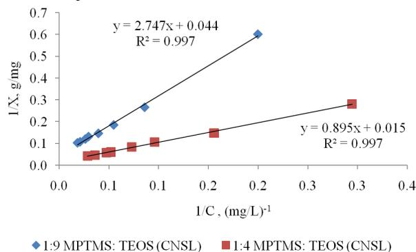
Figure 8. Langmuir plot for lead adsorption onto TSC prepared using CNSL as structure director.
