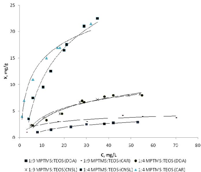
Figure 7. Equilibrium adsorption isotherms for lead onto TSC materials.
