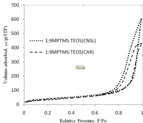
Figure 4. Adsorption-desorption isotherms of the 1:9MPTMS:TEOS(CNSL) and 1:9MPTMS:TEOS(CAR).
