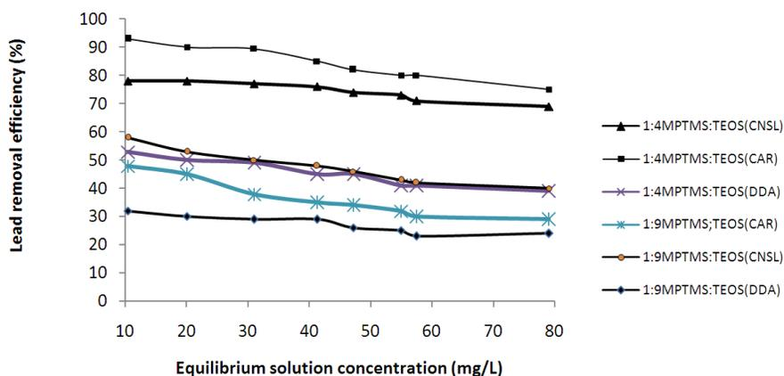
Figure 6. Removal efficiency of Pb(II) ions according to initial concentration.
