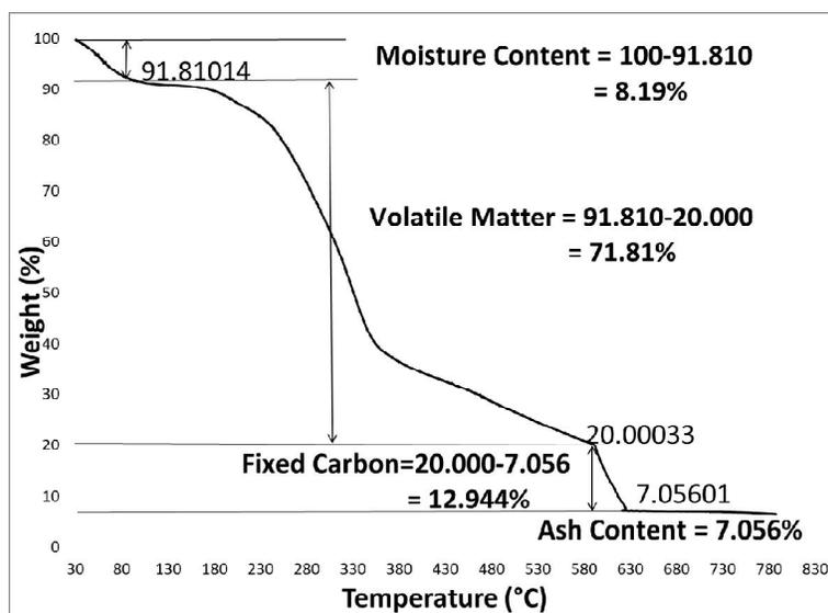
Figure 2. Percentage weight loss of DPF with temperature.
