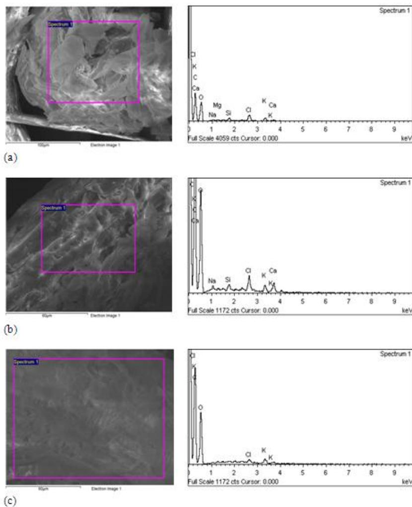
Figure 3. EDX images and elemental composition of (a) Ajwah, (b) Sukariah and (c) Jeddah.
