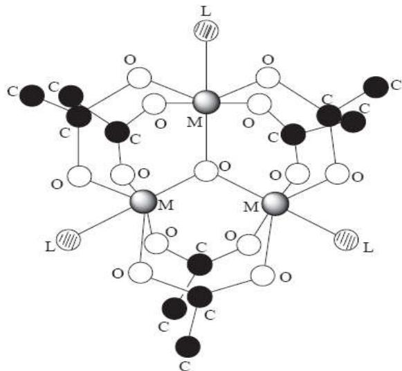
Figure 1. Schematic representation of the oxo-centered trinuclear clusters structure  $[M_3O(RCOO)_6(L)_3]^{2+}$ .
