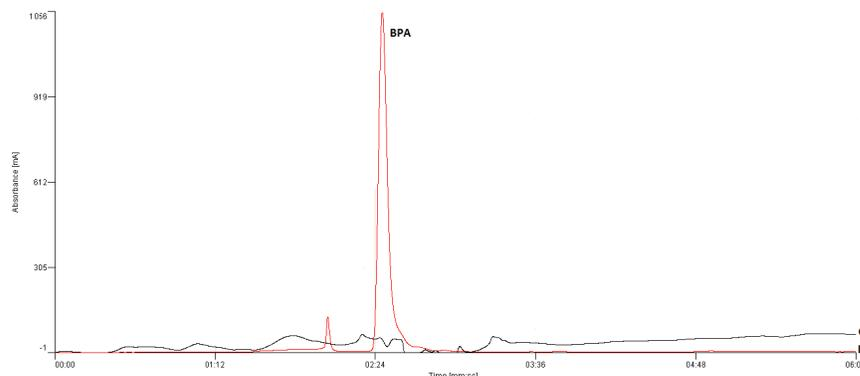
Figure 3. Chromatograms obtained at optimum extraction condition of real samples: A) direct injection of drinking water spiked with  $50 \mu\text{g.L}^{-1}$  of BPA; B) injection of drinking water spiked with  $50 \mu\text{g.L}^{-1}$  of BPA after PT-SPE extraction; C) direct injection of filtered peach juice spiked with  $50 \mu\text{g.L}^{-1}$  of BPA. D) injection of filtered peach juice spiked with  $50 \mu\text{g.L}^{-1}$  of BPA after PT-SPE extraction.
