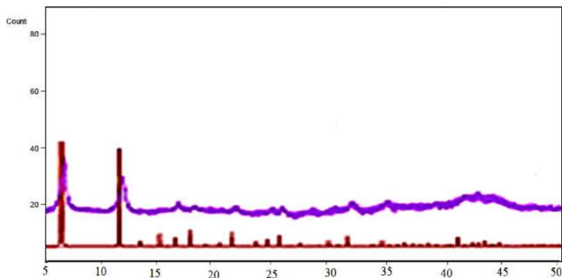
Figure 1. XRD patterns of the Co-MOF synthesized.
