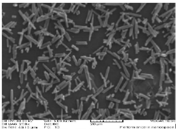
Figure 2. SEM image of the synthesized Co-MOF.
