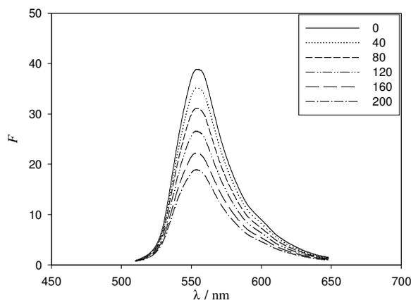
Figure 1. Fluorescence emission spectra of rhodamine 6G (from top to bottom, the concentrations of  $\text{Fe}^{3+}$  were: 0, 40, 80, 120, 160, 200  $\mu\text{g/L}$ , respectively).
