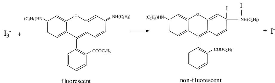
An addition reaction occurs between  $\text{I}_3^-$  anion and R6G at the C=N double bond, because of the heavy atom effect from iodine atom [13], the fluorescence of R6G is quenched.
