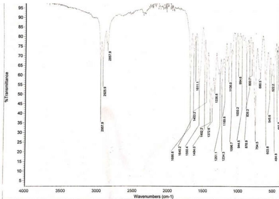
Figure 2. FT-IR spectrum of complex 1.
