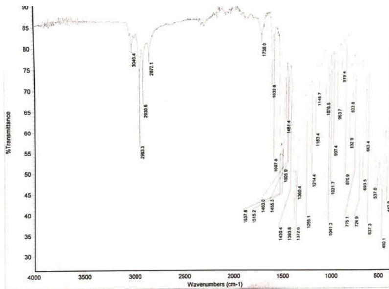
Figure 3. FT-IR spectrum of complex 2.
