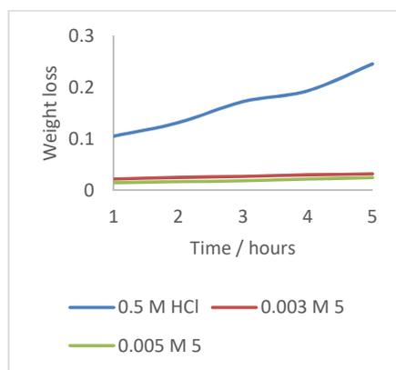
Figure 5. Weight loss of **5** against immersion time at 298 K.
