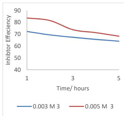
Figure 4. Inhibitor efficiency of **3** against immersion time at 298 K.
