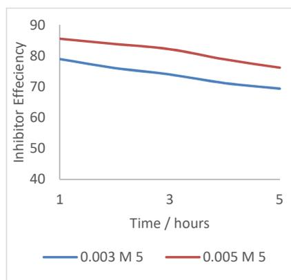
Figure 6. Inhibitor efficiency of **5** against immersion time at 298 K.
