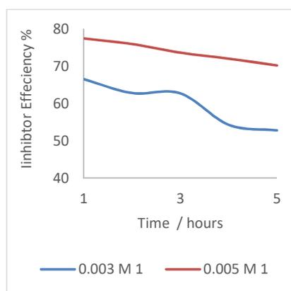
Figure 2. Inhibitor efficiency of **1** against immersion time at 298 K.
