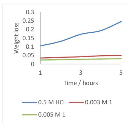
Figure 1. Weight loss of **1** against immersion time at 298 K.
