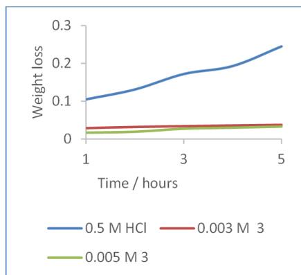
Figure 3. Weight loss of **3** against immersion time at 298 K.
