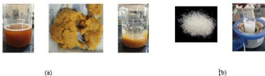
Figure 2. Preparation of membrane components: (a) watermelon rind slurry and (b) PVA solution.
