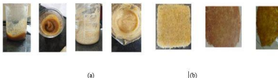
Figure 3. Fabrication of biopolymer membrane: (a) homogeneous blending and (b) casting and drying.
