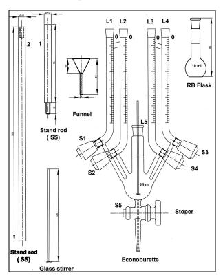
Figure 1. Sketch diagram of the semimicro volumetric kit: Stopcock model.
