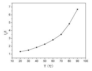
Figure 3. Effect of temperature on the fluorescence intensity of the sensor.
