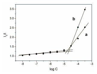
Figure 5. The calibration curve for Fe<sup>3+</sup> determination (a) the sensor used in this experiment and (b) the sensor fabricated by another grape skin.
