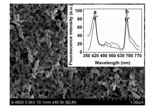
Figure 1. SEM micrograph of the inner surface of grape skin. Inset: fluorescence excitation (a) and emission (b) spectra; a, b: the grape skin-based sensor blank; a', b': adding  $5.0 \times 10^{-5}$  M Fe<sup>3+</sup> to the system.
